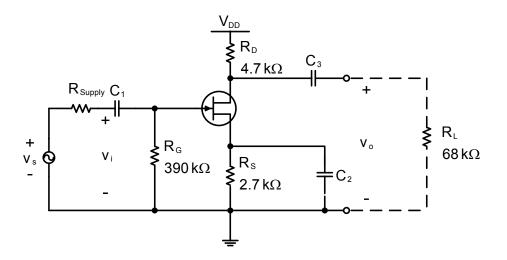
Q4. The JFET in the following diagram has  $V_p = -3$  V and  $I_{DSS} = 9$  mA. Calculate the value of all the resistors so that  $V_G = 5$  V,  $I_D = 4$  mA and  $V_D = 11$  V. The design has 0.05 mA flowing through the voltage divider.
