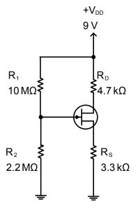
Q3. Calculate the voltage gain and the input and output impedances for the common source circuit shown below.  $R_{GS} = 1000 \text{ M}\Omega$ ,  $g_m = 4000 \mu \text{S}$  and  $r_{ds} = 80 \text{ k}\Omega$ . Determine the voltage gain if  $C_2$  is absent.
