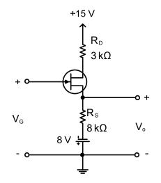
Q2. Given the drain to ground voltage is equivalent to 5 V for the circuit below. Calculate  $I_D, V_{GS}, V_{DS}$  and  $V_S$  for this circuit.
