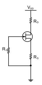
**Q8.** Referring to the following circuits, determine the DE MOSFET's mode of operation (depletion, enhancement or zero). Give explanation to your answer. Assume  $R_G$  is very large that the current flowing through it can be neglected resulting in  $V_{RG} \approx 0$ .
